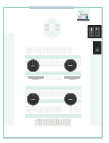
Attero Tech by QSC unD6IO-BT network audio wallplate features Bluetooth audio connectivity into the system Attero Tech by QSC Axon C1 provides simple audio controls (volume, playback controls)
