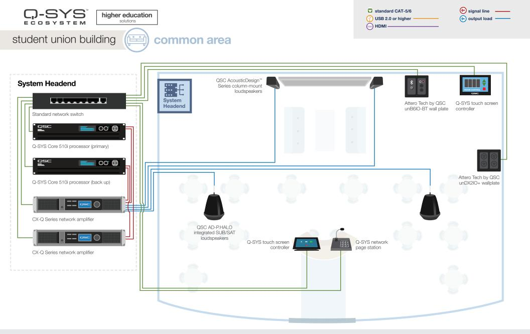
Redundant Q-SYS Cores provide AV&C processing and CX-Q Series amplifiers provide amplification for café, common area and book store Attero Tech by QSC network audio wallplates act as analog audio on-ramps into the Q-SYS Ecosystem AcousticDesign<sup>™</sup> Series AD-P.HALO provides an integrated SUB/SAT loudspeaker system for an elevated background music experience for students
