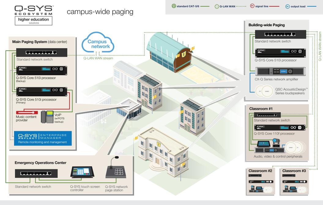
Redundant Q-SYS Cores processors for wide-area paging and BGM functionality User paging via VoIP or POTS Each individual building has a dedicated Q-SYS Core for smaller classroom processing and local paging.
